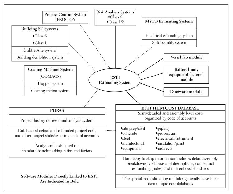
Figure 2-Cost Estimating Systems Diagram
